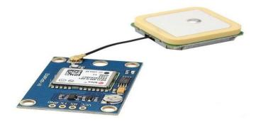
Figure 2. GPS Module (NEO-6M)
