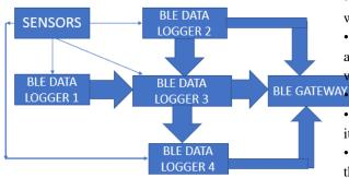
Fig 3. Block diagram of Development of Bluetooth Low Energy based Mesh Network Logger.
