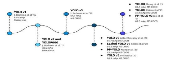
In this project, we have used YOLOv3. YOLOv3 was released in 2018 and further improved the accuracy and speed of the algorithm. It introduced several new features such as multi-scale prediction, feature concatenation, and spatial attention. YOLOv3 achieved an average precision of 87.4% on the COCO dataset. This technique focuses on object recognition and speed of detection without achieving absolute object localization. *Object detection in YOLOv3*:
