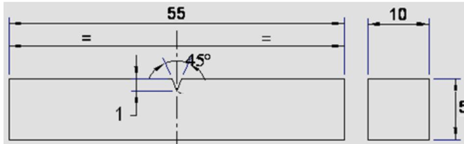
**Dimension view of the impact testing specimen.**
